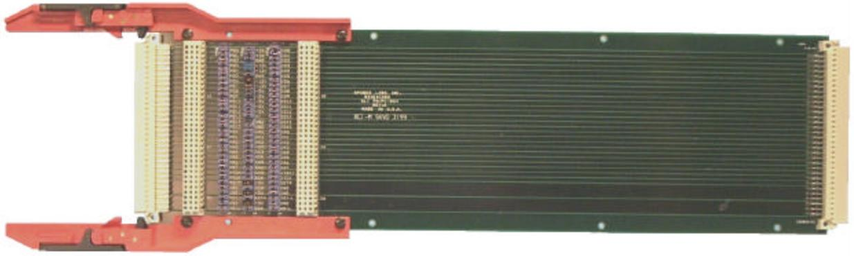
The MITC *FALCON* Extender Card (EXT1) was specifically designed to enable the user to run tests while the unit is in operation.
