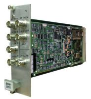
The BSM1 accepts analog PCM data from one of four user selected inputs. It then extracts the data from a potentially perturbated noisy environment, reconstructs a coherent clock along with the recovered data signal. The output of the bit synchronizer is TTL data and clock as well as a bipolar representation of the data that is suitable for application to a tape recorder. The performance of the bit synchronization process is within 1dB of theory.
