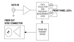
IOC501TX (TRANSMIT) BLOCK DIAGRAM
