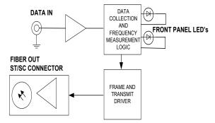
IOC501TX (TRANSMIT) BLOCK DIAGRAM
