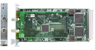
daughter card, mounted to the main or mother card, which implements an unchannelized E2 or E3 interface structure. The interface type is automatically detected.
