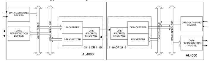
These interfaces are designed as point-to-point data-link packetizer and depacketizer devices. The E2LNK and E3LNK modules support system configurations where it is necessary to share data between system nodes that are separated by cable distances of up to 1300 feet.
