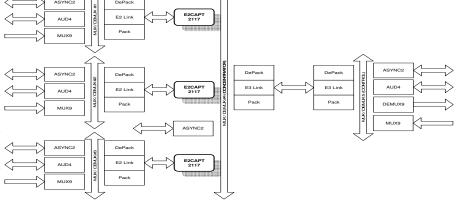
These modules are designed as point-to-point data-link packetizer and depacketizer devices for data concentration applications. The E2CAPT modules support system configurations where the distance between system nodes is up to 1300 feet.
