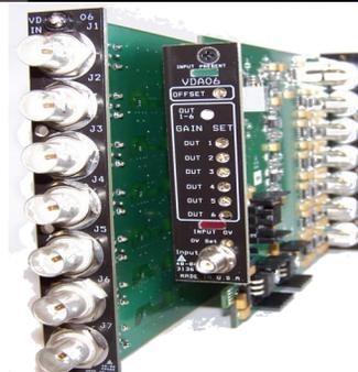
The Apogee Labs RF04/RF06 is an Interfacer II module that is designed to accept a single wide-band signal and reproduce it on four or six independent gain controlled outputs. The module presents its controls and indicators and a test-point connector on its front panel. The signal input and four/six outputs are located on the module rear panel. All rear panel connectors are BNC type. The front panel connector is SMA type.
