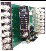
The Apogee Labs RF04/RF06 is an Interfacer II module that is designed to accept a single wide-band signal and reproduce it on four or six independent gain controlled outputs. The module presents its controls and indicators and a test-point connector on its front panel. The signal input and four/six outputs are located on the module rear panel. All rear panel connectors are BNC type. The front panel connector is SMA type.
